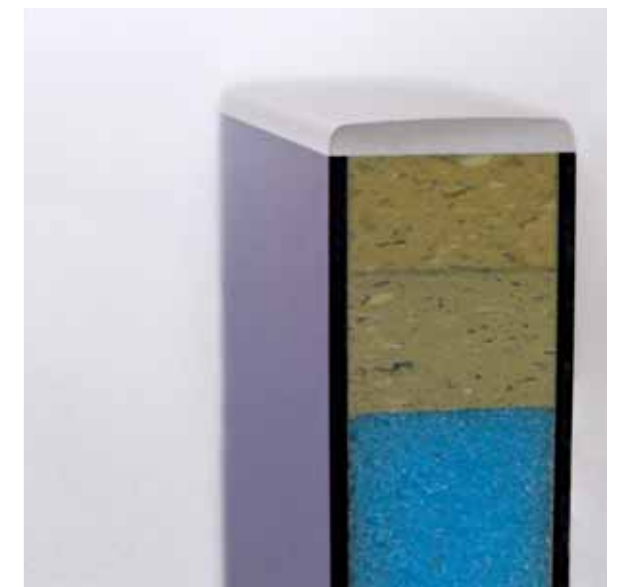
Water-resistant door leaves Non-rebated or as a deeper flat panel, can also be used for existing standard door frames. Rigid foam core with reinforced edges, covered with 3mm HPL Compact on both sides, surrounded by an impact-resistant PUR edge.
